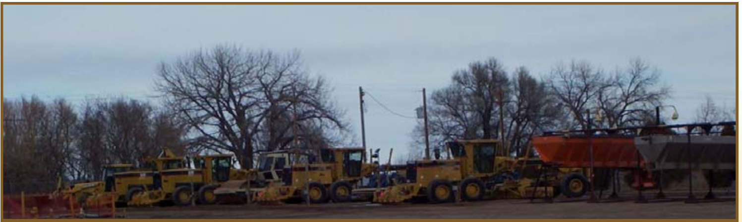
Larimer County owns 23 motor graders. These units are used for road maintenance and are located throughout the county in different departments. This type of equipment burns about 43 gallons of diesel in an 8 hour shift. Photo: Darrell St Peter
